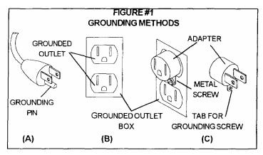
If repair or replacement of the cord or plug is necessary, do not connect the grounding wire to either flat blade terminal. The wire with insulation having an outer surface that is green with or without yellow stripes is the grounding wire.
